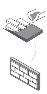
When the InBrick panel is erected, the VersaLiner® is stripped from the face and the panels are cleaned. The end result is an InBrick concrete precast panel with an InBrick cast façade.
