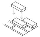
After reinforcing is placed, concrete is poured over the configuration and finished in the normal manner.
